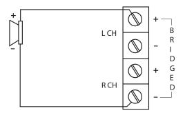
**Note:** The A1004 amplifier connections are the same as shown above, except that there are outputs for Front and Rear speakers.
